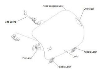
The bolt latch is installed at the front end of the luggage doors. When the button on the latch is pressed, a spring in the latch unlocks the bolt from the door structure and rotates the button 180 degrees to show that it is unlocked. The lower part of the button is orange to make the unlocked position visible.
