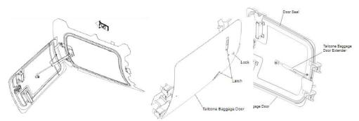
To open the door, the lock must be unlocked and both latches must be released. There is a pneumatic spring that extends to help keep the door in the open position.
